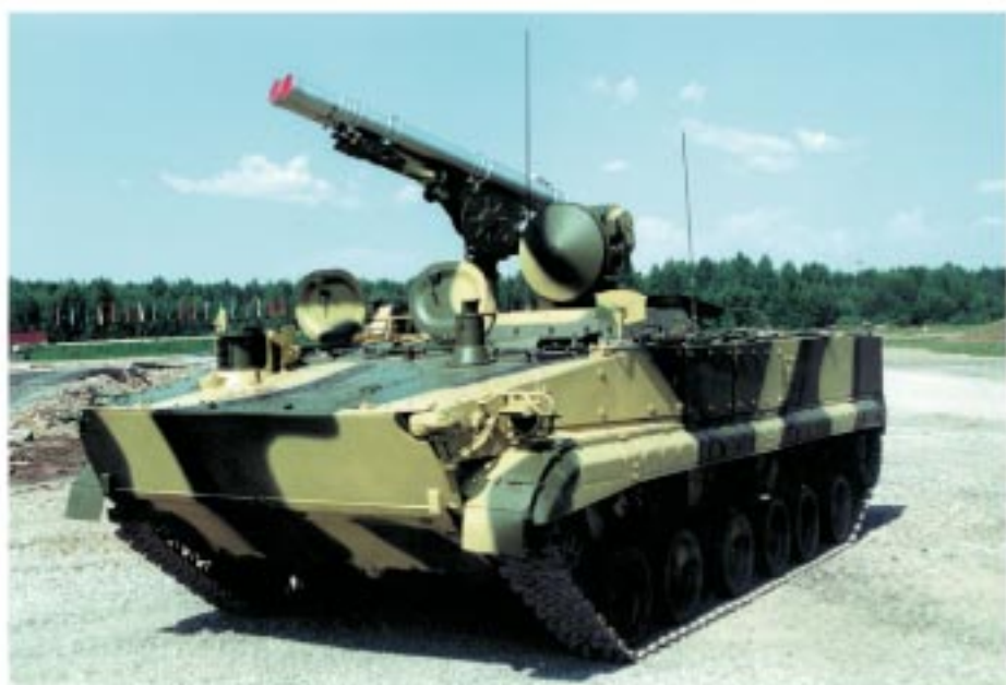
Khryzantema missile system on the basis of the BMP-3 chassis
